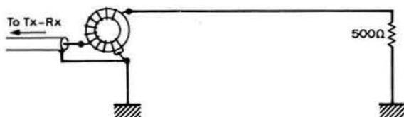
Fig 6. G3SRO's terminated long-wire aerial with ferrite broadband matching transformer
